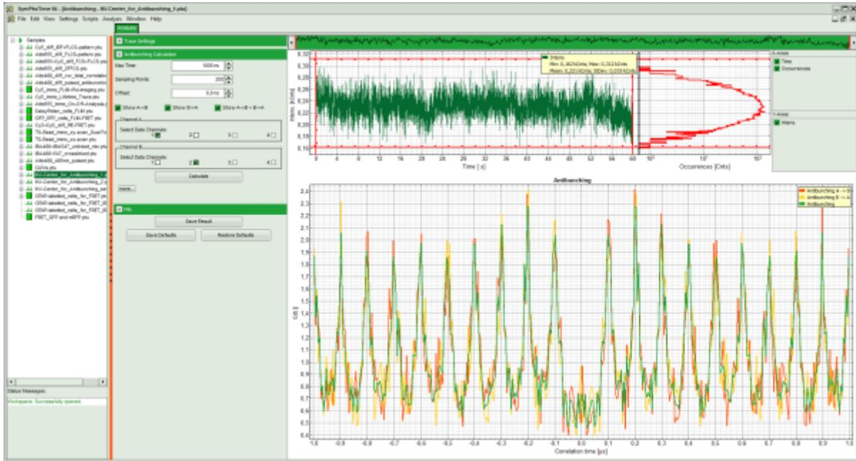
**Note:** If the cable lengths are different for both detectors, photons simultaneously registered at the detectors arrive a different times at the photon counting TCSPC unit. Consequently, a systematic shift of the red and the yellow curve is observed. For compensation adjust the “Offset” parameter. It automatically moves the red and yellow curve to the correct position. Press “Calculate” again to recalculate the correct antibunching curve.
