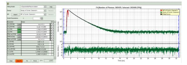
**Response:** The TCSPC curve is fitted. A  $\chi^2$  close to 1 and nicely spread residual indicate a sufficiently good fit.
