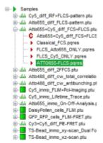
• Now the FLCS autocorrelation curve for the second dye (Cy5) must be calculated. Therefore, select this pattern (corresponding to ~0.8 ns) in the FLCS main window and press "Calculate".
