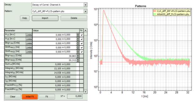
• Press "Initial FIT" to fit these patterns to the decay of the FCS measurement.
