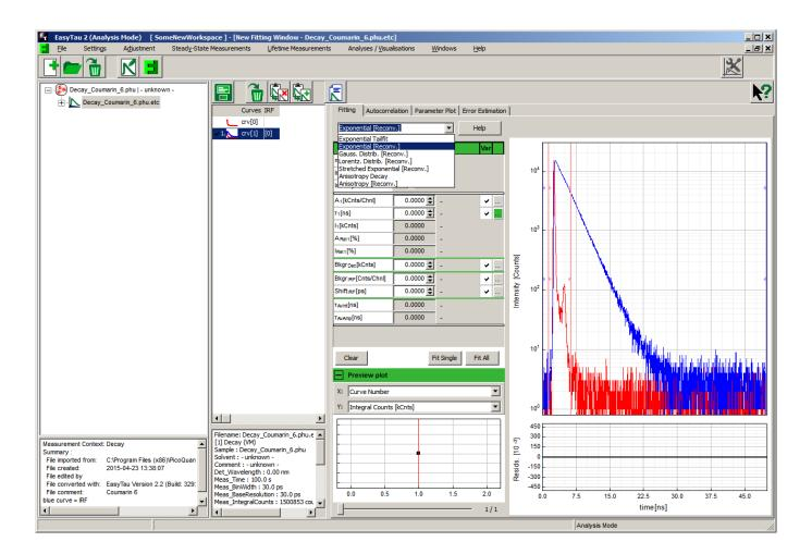
If necessary, change the time axis limits by dragging the appropriate vertical sliders in the plot. There are dedicated sliders for both IRF and decay curve time ranges. Pressing the "Fit Single" button performs a fully automated fit of a single exponential decay model:
