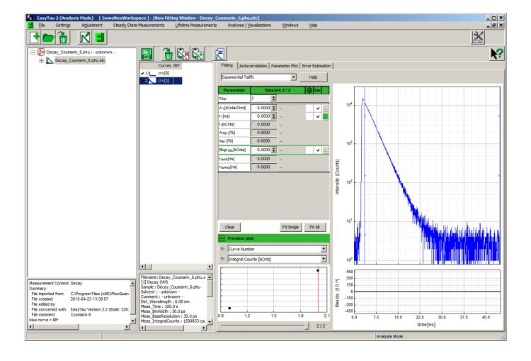
Clicking on (selecting) crv[0], the first histogram, the IRF in this particular case, updates the plot. Now, a right-click on crv[0] opens a context sensitive dialog, where the "Curve type" can be changed from "Decay" to "IRF".
