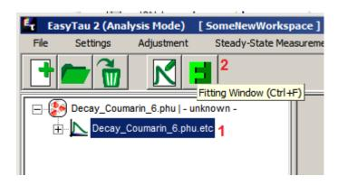
The last curve in the container, crv[1], a decay curve in this case, is displayed. The default fitting option is "Exponential Tailfit". In order to perform a reconvolution fit, we need to select and then assign a curve as an IRF and then change the fitting modality.
