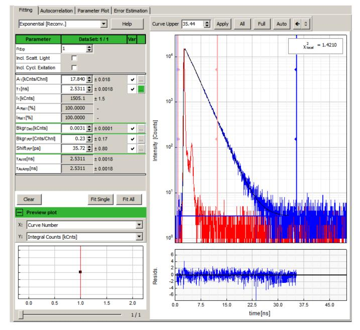
This simple model is entirely appropriate for this particular decay curve. However, the complexity of the model can be increased by adding more exponential terms ( $n_{Exp}$ ) or activating the correction for scattered light or cyclic re-excitation. The mathematical formulas and definition of terms is available by pressing the "Help" button inside the fitting dialog. It is possible to fix any parameter of the fitted model by removing the corresponding tick in the "Var" column.
