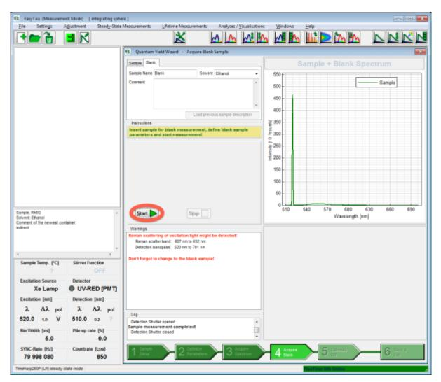
• After the acquisition of the blank spectrum has finished click the "Calculate QY" button.
