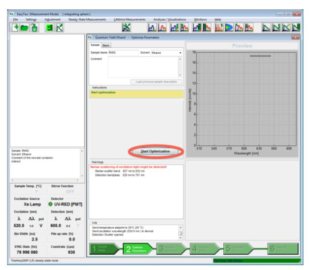
• After the optimization has successfully finished, click the "Acquire Spectrum" step and review the measurement conditions. If necessary tweak the acquisition time.
