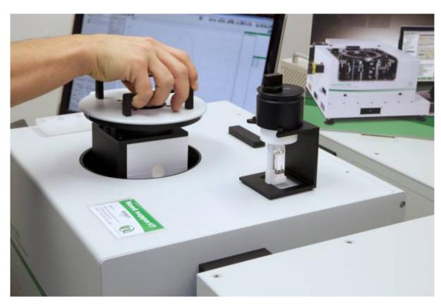
• Mount the integrating sphere carefully. Make sure you do not hit any optical elements inside the FluoTime 300. The integrating sphere assembly has an indexed lid to ensure proper orientation.
