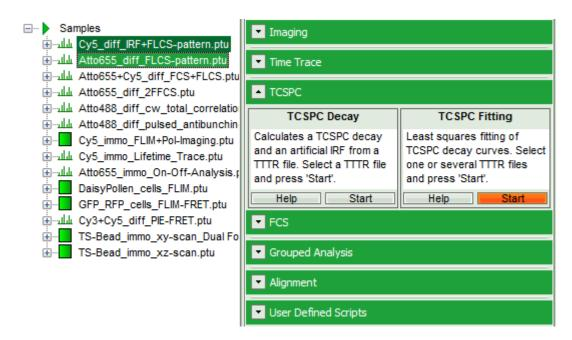
**Response:** The TCSPC fitting window is opened and the TCSPC histograms of both files are loaded. The TCSPC histogram from the file "ATTO655\_diff\_FLCS-pattern.ptu is marked in green, indicating that it is the active file. Under decay data all files are listed, the active file is always highlighted in green.
