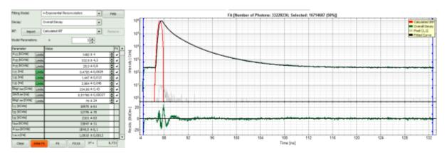
• For fitting of a 3-exponential decay into every pixel, a certain number of photons is necessary. How many, is determined by the complexity of the model. In order to check whether the photon number is sufficient for the model suggested, click on an average pixel of interest in the FLIM image.
