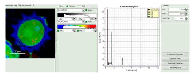
• The three lifetime components can be displayed in a false color scale. Therefore switch the display to "RGB" and adapt the intensities of each color as preferred.
