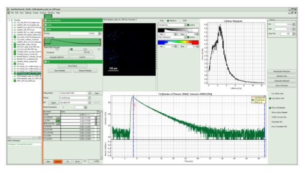
• To enhance the lifetime and intensity contrast, set in the image the intensity from 1 count to 30 counts and the lifetime from 0 to 5 ns.
