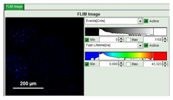
• Set the intensity scale from 0 counts - 200 counts and the lifetime scale from 0 to 5 ns.
