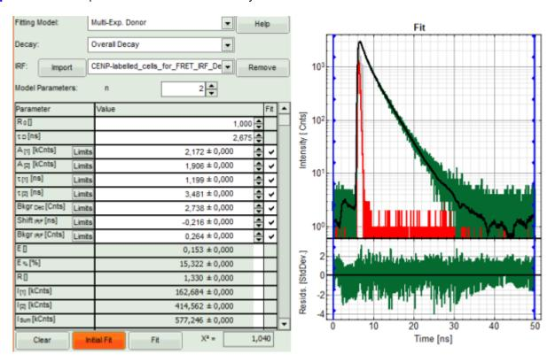
• In the Fitting panel, set the parameters Bkgr<sub>Dec</sub>, Shift<sub>IRF</sub> and Bkgr<sub>IRF</sub> constant by removing the mark. Set the background of the decay to 0.
