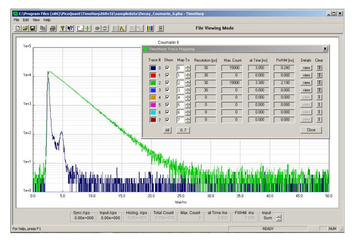
Trace #0 shows the IRF, Trace #2 is the decay curve. The other data blocks are empty. Both Trace #0 and #2 will be imported into a single .etc data container. This will make the data analysis easier. In general, such a .phu file may contain many more histograms.
