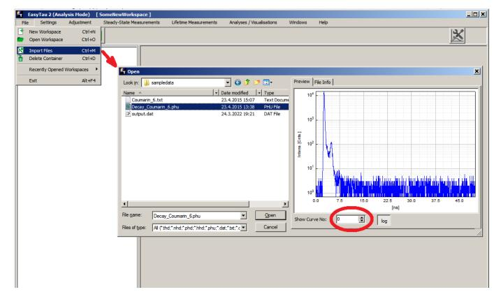
The file selected above is a sample data file, Decay\_Coumarin\_6.phu installed during the installation of the native TimeHarp260 software. This file contains two histograms: an Instrument Response Function (IRF) and a decay curve of Coumarin6 dissolved in ethanol. During file import, before pressing the Open button, it is possible to preview and step through the data content of selected file using the control elements on the right hand side of the dialog.
