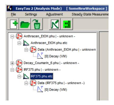
Unlike Decay\_Coumarin\_6.phu containing two histograms, both Anthracene\_EtOH.phu and IRF375.phu contains only one histogram. These two measurements actually belong to each other. In order to perform reconvolution fitting of the Antracene decay, the corresponding IRF measured at 375nm excitation wavelength will be needed.
