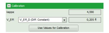
**Note:** By default, V\_Eff\_D calculated from the diffusion constant is chosen as calibration value. If the reference were the concentration, the assignment can be changed in the "Calibration" drop down menu (see image above).
